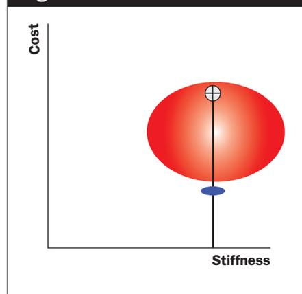
Instead of putting 24 oz/sq yd of biaxial down—to match the properties of the carbon—we'll put down 44 oz/sq yd. The cost and weight increase.
